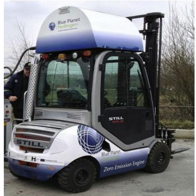
Forklift truck equipped with a H 2 ICE, part of the demonstration activities within the Hydrogen Region Flanders South-Netherlands project
