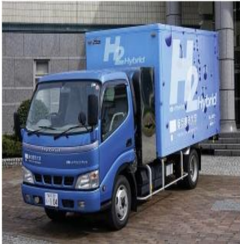
Hybrid light duty truck equipped with a 4 L 91 kW hydrogen engine , demonstrated by Tokyo City University
