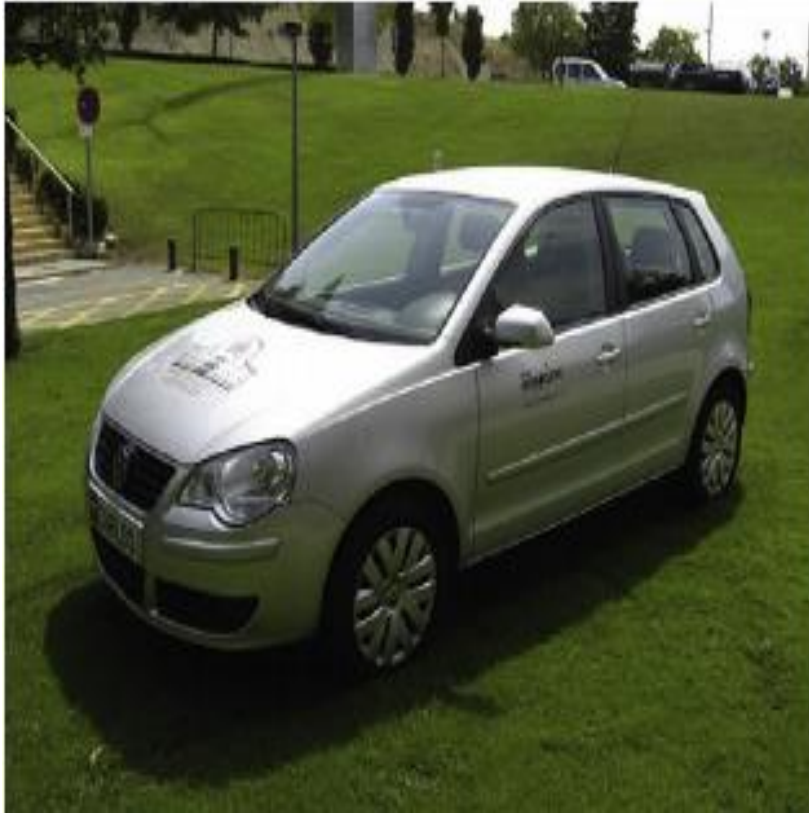
Bi-fuel (gasoline/hydrogen) VW Polo demonstrated by the University of Navarre
