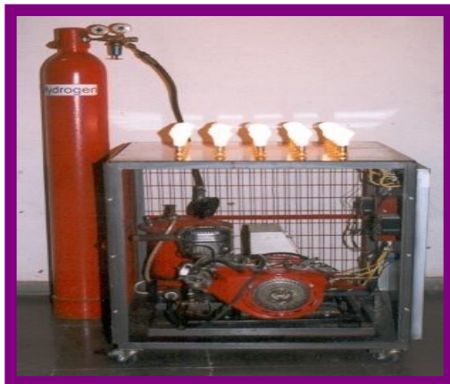
TOTAL HYDROGEN S.I. ENGINE GENSET USING ELECTRONIC FUEL INJECTION SYSTEM
